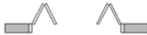
Bifold Doors - Indicates bifold doors and direction of operation, like closet doors.
