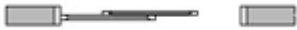
Sliding Door - Symbol for sliding glass door in a solid wall indicating which panel slides.
